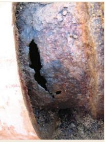
PHOTO 2 Ductile iron pipe joint failure (10 years).
