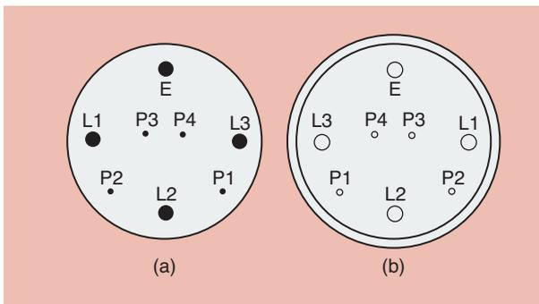
**FIGURE 4.** The power plug and socket pin assignment. (a) The plug/ship inlet face and (b) the socket-outlet/ship connector face. E: earth; L1: phase 1–A–R; L2: phase 2–B–S; P1: pilot 1; P2: pilot 2; P3: pilot 3; P4: pilot 4.
