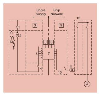
**FIGURE 1.** An LVSC block diagram: the 1) primary breaker, 2) substation transformer, 3) LV switchgear, 4) main breaker, 5) feeder breakers, 6) feeder cables to power receptacles, 7) plug and receptacle assemblies, 8) plug with a flexible cable, 9) ship onboard shore power panel, 10) ship-side circuit breaker, 11) optional ship onboard transformer, 12) synchronizing breaker, and 13) neutral resistor disconnect switch. G: ground.
