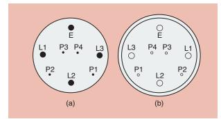
**FIGURE 4.** The power plug and socket pin assignment. (a) The plug/ ship inlet face and (b) the socket-outlet/ship connector face. E: earth; L1: phase 1–A–R; L2: phase 2–B–S; P1: pilot 1; P2: pilot 2; P3: pilot 3; P4: pilot 4.
